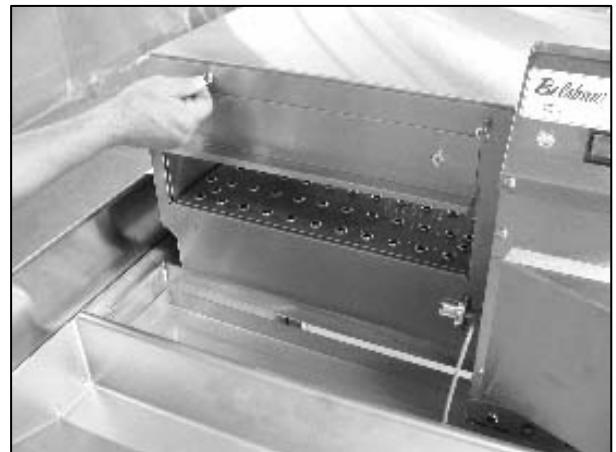
21. Install the outfeed end cover same as the infeed.
